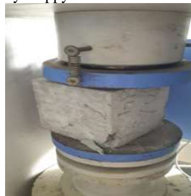
Fig 3.6. compressive strength of cube
